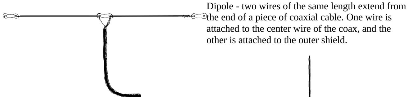
Dipole - two wires of the same length extend from the end of a piece of coaxial cable. One wire is attached to the center wire of the coax, and the other is attached to the outer shield.
